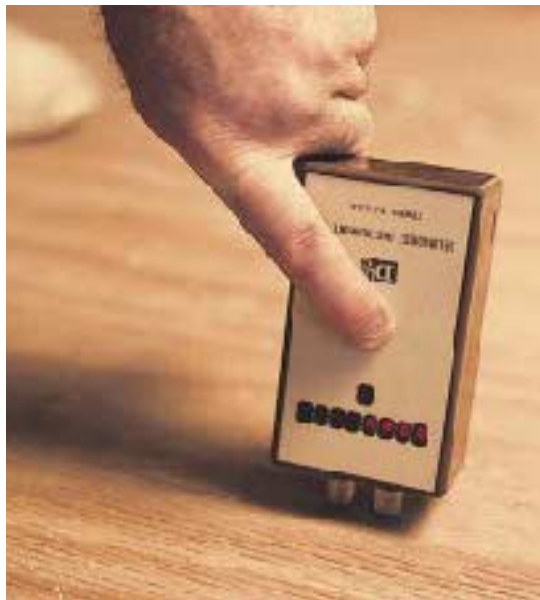
Figure 3. Using a moisture meter is the only accurate way to check for excessive moisture in subfloors and finish flooring strips. A pocket-size meter costs less than $200 and is an essential tool for good wood flooring installations.
