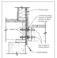
A properly-flashed deck ledger protects the house rim joist from water damage. The drip-edge on the metal flashing prevents moisture from wicking into the sheathing, and the metal spacers behind the ledger allow for air circulation. centers as spacers, then bolted the ledger through them to the wall. We bevel the tops of the blocks to drain water and we caulk, too, but keep the nailing of the blocks to a minimum.
