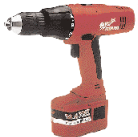
Figure 5. Milwaukee's new 14.4-volt hammer drill (shown above) and T-handle driver/drill both use a reversible 2.4 Ah NiCad battery. Changing the battery orientation alters the tool's balance, making it more comfortable to use in various positions.
