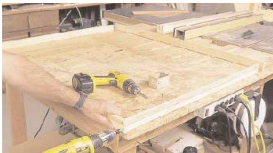
Figure 4. The author preassembles picture-framed extensions in his shop. All four corners are screwed to the keep the joints tight.
