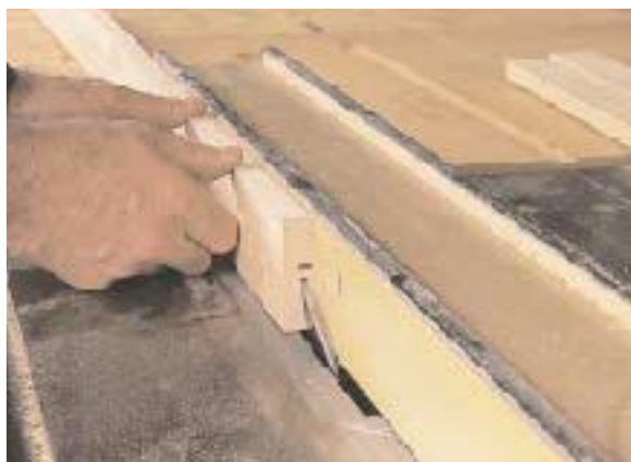
Figure 3. A back-rabbeted extension can be milled on site in two passes with a table saw. The bevel cut begins at the corner of the stock and meets the shoulder cut about 1 inch from the window-side edge. Back-rabbeted extensions can be fastened with a nail gun before the window is installed.
