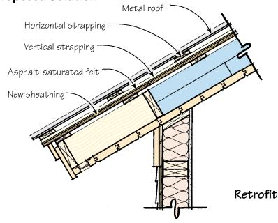
have been prevented from leaking through the joints between the T&G boards, as long as the plastic were properly overlapped, as is done for roofing felt. However, that water would have been trapped by the 2-by blocking at the eaves and it could eventually have penetrated the walls below or rotted nearby lumber, which would be an invitation for carpenter ants.
