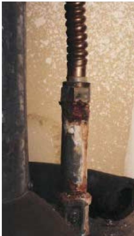
Figure 1. Water with low pH levels or high CO 2 content, often referred to as aggressive water, can prematurely wear out copper piping (left). Thermal-galvanic corrosion, caused by a variety of factors, usually damages hot water pipes first (right).
