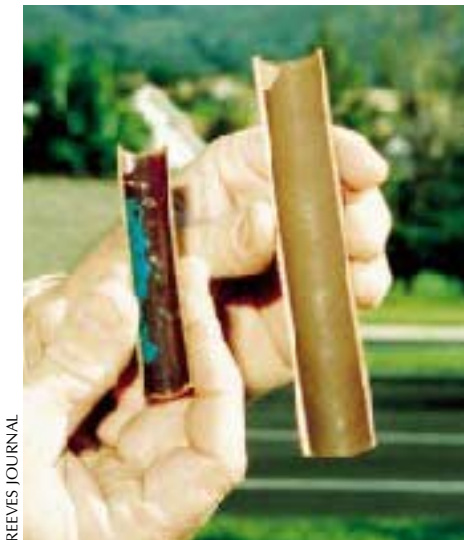
Figure 1. Water with low pH levels or high CO 2 content, often referred to as aggressive water, can prematurely wear out copper piping (left). Thermal-galvanic corrosion, caused by a variety of factors, usually damages hot water pipes first (right).
