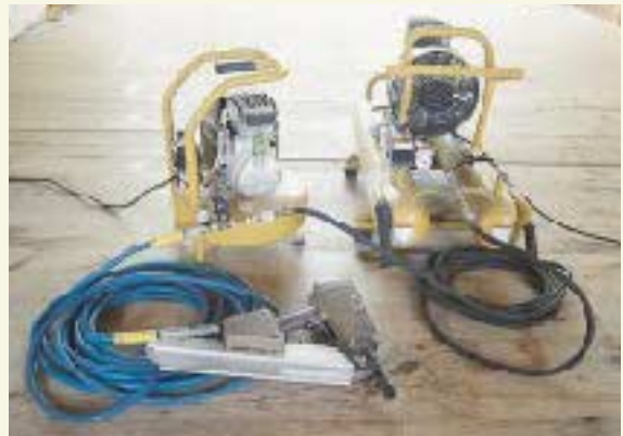
Daisy chain. The author connects these two portables together to get the performance of a larger compressor.
