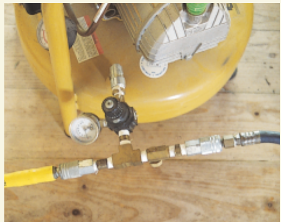
B. T-fitting. The hose leading from the first compressor and the hose leading to the nailer join at this T-fitting.
