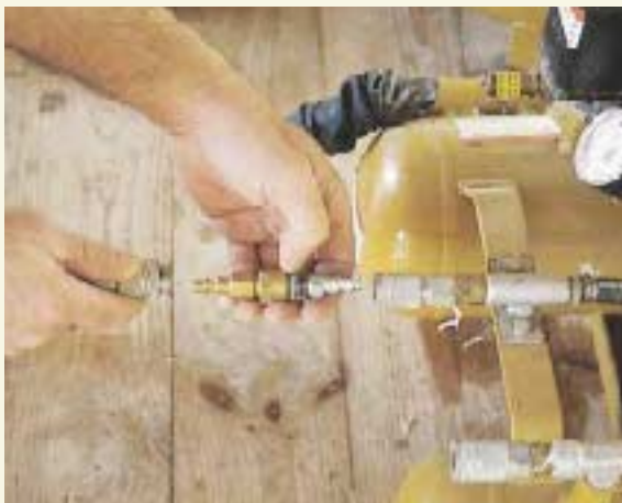
A. Coupling. At the first compressor in the daisy chain, the author uses this fitting to connect a hose leading to the next compressor.
