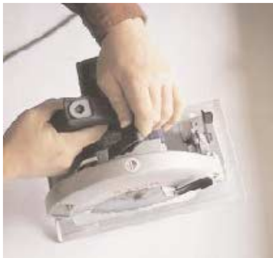
Figure 2. The blade guard on the Bosch retracts by means of a lever mounted next to the handle high on the blade housing. The action is smooth and keeps your fingers away from the blade.
