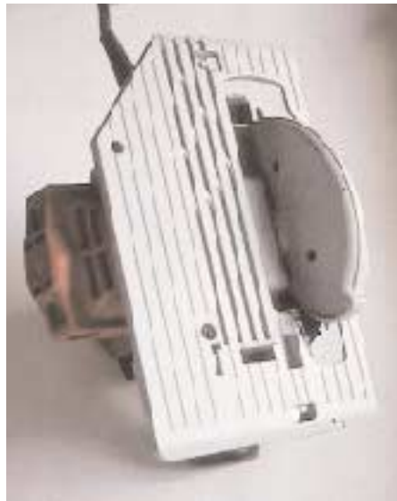
Figure 6. Most shoe damage occurs on the rear inside corner, so Milwaukee cut the corner off altogether. Like a few others, this shoe is also grooved to reduce friction.
