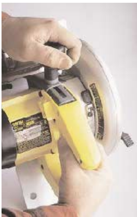
Figure 4. The smooth-acting DeWalt 364 depth adjustment is built into the handle and is locked with a long-necked knob that provides plenty of clearance for your fingers (left). The sturdy ball-joint pivot (above) is mounted at the back of the shoe, so your hand remains in a comfortable position even on shallow cuts.
