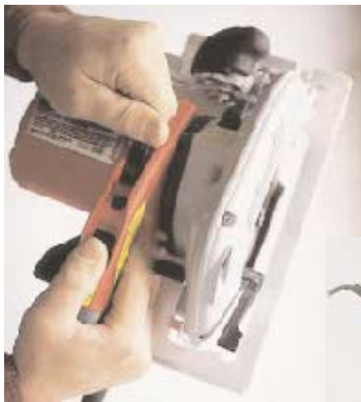
Figure 1. The position of the handle on the Milwaukee 6390 can be adjusted by releasing a lever on top (left). The handle pivots through eight positions (below), making the saw easier to grip at shallow depth settings or when reaching across full sheets of plywood.
