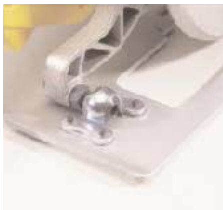
Figure 4. The smooth-acting DeWalt 364 depth adjustment is built into the handle and is locked with a long-necked knob that provides plenty of clearance for your fingers (left). The sturdy ball-joint pivot (above) is mounted at the back of the shoe, so your hand remains in a comfortable position even on shallow cuts.
