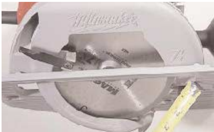
Figure 3. On the Milwaukee 6375-20, when setting the bevel to 45 degrees at full depth, a cam on the cast shoe engages and retracts the blade guard about 1 inch — just enough to get the cut started smoothly. The Milwaukee 6390, both DeWalts, the Bosch and the Skil do the same thing by means of a cam-like extension on the arm of the blade guard.
