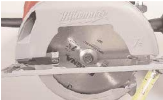
Figure 3. On the Milwaukee 6375-20, when setting the bevel to 45 degrees at full depth, a cam on the cast shoe engages and retracts the blade guard about 1 inch — just enough to get the cut started smoothly. The Milwaukee 6390, both DeWalts, the Bosch and the Skil do the same thing by means of a cam-like extension on the arm of the blade guard.
