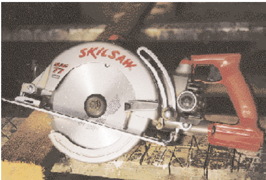
Figure 2. Skil's use of magnesium in the saw body and table shaved a few pounds off its Mag77 worm-drive saw. Although some of the author's crew thought the edges of the redesigned table were too sharp, overall this new worm-drive gained widespread approval.
