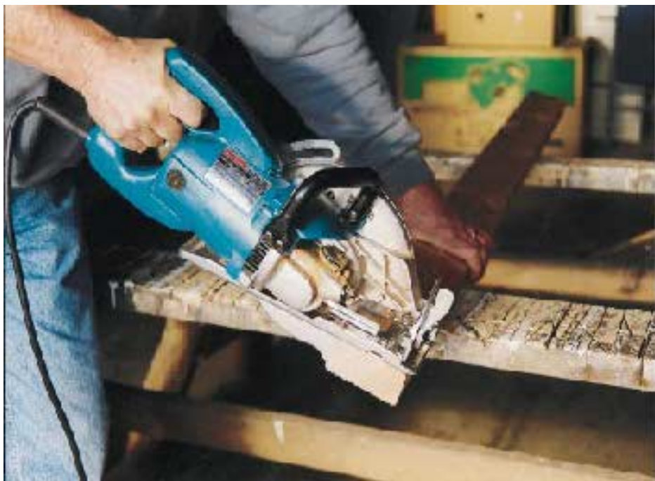
Figure 4. Makita's in-line circular saws feature hypoid gears. The company has eliminated the start-up jump that made the older model so hard to work with. In fact, the author found the 5177B to be the smoothest-starting saw tested.
