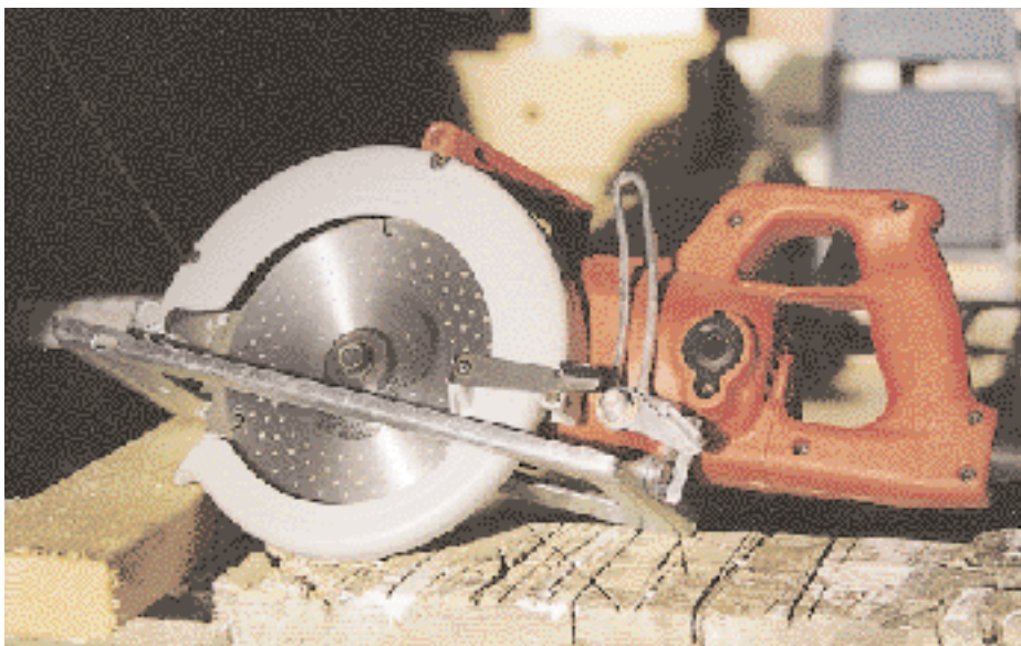
Figure 3. Milwaukee's worm-drive saw was the heaviest saw tested and probably would not be comfortable for all-day use. Undeniably powerful and rugged, the author found a few weaknesses, such as a poorly positioned depth-adjustment arm and a guard that did not retract well on thin end cuts and bevels.
