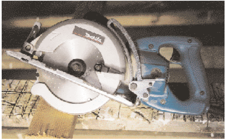
Figure 5. The new Makita in-line framing saws feature good blade guards and a special cut in the table that makes for easy blade alignment.
