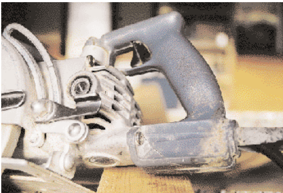
Figure 1. Because of its popularity with West Coast framers, the Skil77 served as the author's benchmark testing tool. Today's Skil77 is still as rugged and dependable as ever, although it's too early to tell whether the handles will crack like they have on the older saw shown here. Also, the guard on the Skil77, although okay, has not been improved over the years.
