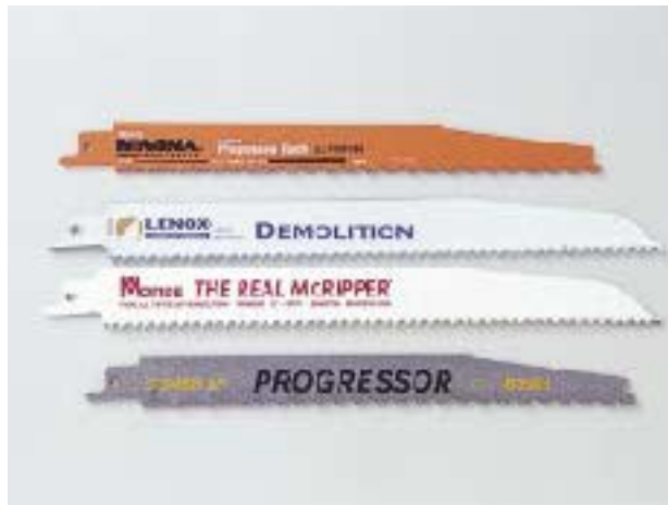
Figure 6. The progressive-tooth all-purpose Magna 90452 blade ate the Nasty Sandwich for lunch, making seven cuts without slowing down. The Lenox 966R and Morse RB96296 each made three cuts. Although the Bosch S3456XF made just one quick cut before slowing significantly, it performed better on its third cut than many blades did on their first.
