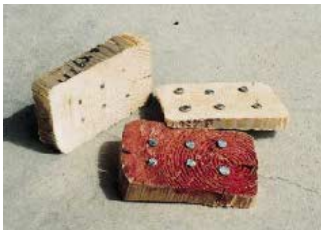
Figure 3. Scraps accumulated rapidly (above) as each blade made multiple cuts through a variety of test materials. Nail-cutting tests were made on Douglas fir 4x6s embedded with six 30-penny nails (right).
