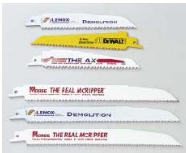
Figure 7. In general, it's easier to make a plunge cut with a short blade than a long one. Despite their added thickness, most of the demolition blades still jumped around too much to be useful, but these six blades made smooth, accurate cuts.
