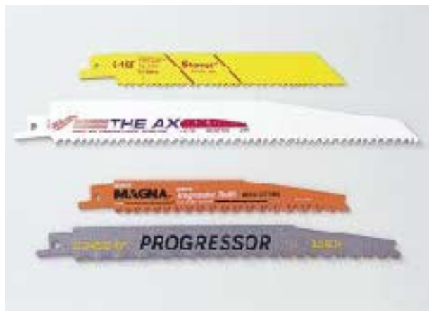
Figure 1. A “variable” tooth design (top two blades) alternates the size and number of teeth per inch across the length of the blade. With a “progressive” tooth pattern (bottom two blades), teeth grow in size from the shank to the tip. Designed to enable cuts in a wider variety of materials, the more aggressive tooth angle on these blades makes for faster cuts.
