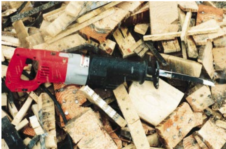
Figure 3. Scraps accumulated rapidly (above) as each blade made multiple cuts through a variety of test materials. Nail-cutting tests were made on Douglas fir 4x6s embedded with six 30-penny nails (right).
