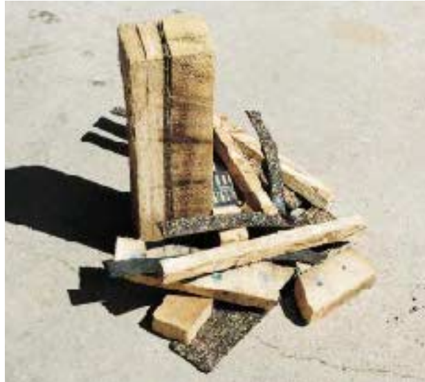
Figure 5. To simulate heavy roof demolition, blades had to cut through the “Nasty Sandwich” — two asphalt shingles sandwiched between two layers of 1/2-inch OSB, a truss plate, and a 2x10 with five 16-penny nails driven into the end grain.
