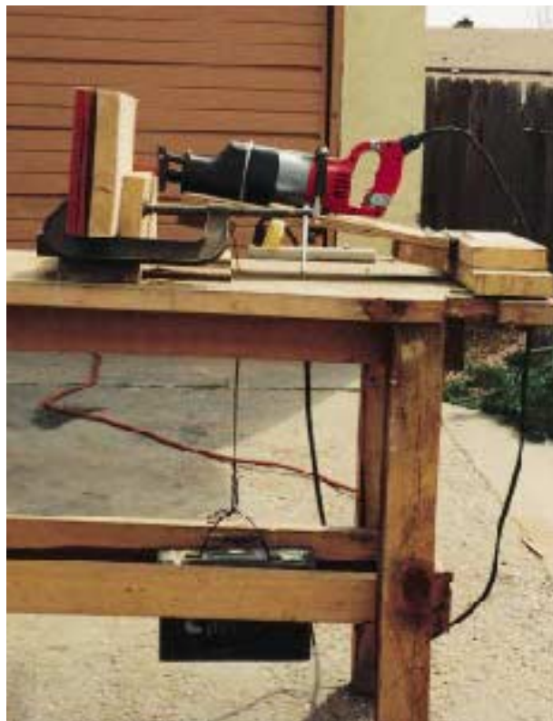
Figure 2. Blades were tested at high speed in a Milwaukee Super-Sawzall bolted to a hinged table that ensured a consistent range of motion. A hanging weight applied a consistent 28 pounds of pressure during each cut.
