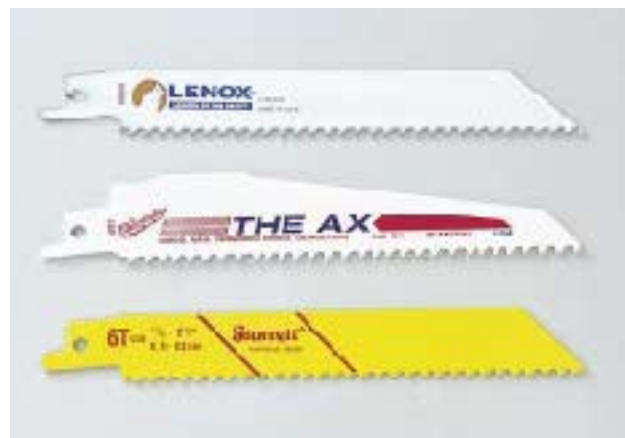
Figure 4. The top-performing nail-cutting blades were the Lenox 606R, which reached the test limits after 35 cuts but never actually wore out; the Milwaukee Ax 5021, which cut accurately without bending; and the Starrett B66, which never slowed down through 22 cuts but was very flexible and ultimately snapped.
