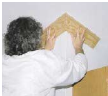
Figure 2. The Miter Finder compensates for out-of-square corners. After entering the crown molding spring angle, hold the tool against the corner (top). A push of a button displays the miter angle; another push displays the bevel. Test cuts produced perfect paint-grade joints (bottom).
