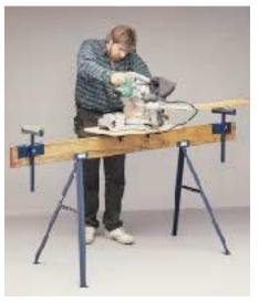
stored behind a truck seat. At the job site, the Workcenter goes together quickly, using a piece of 2x lumber as the cross beam.
