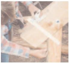
The square blade is 11/2 inches wide, which works out perfectly for plate and joist hanger layout, and has handy roof layout tables written right on it. To top things off, the fixed arm of the square has a built-in spirit vial, so the square can be used like a torpedo level — or to find the pitch of an existing roof.
