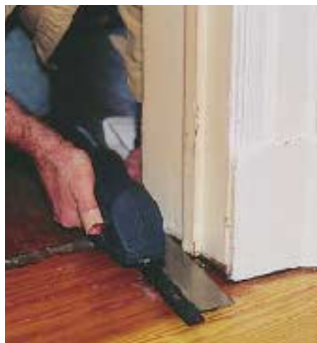
Figure 1. The Finecut Power Handsaw's flush-cutting blade makes it easy to trim door jambs and casing to allow room for flooring.
