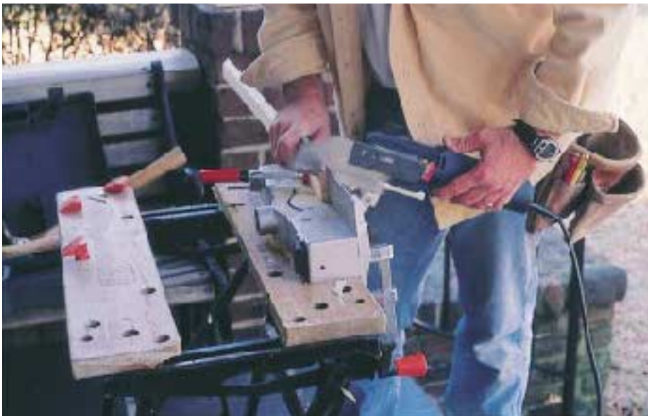
Figure 2. One bolt is all it takes to convert the 1640VS from freehand saw to power miter box.
