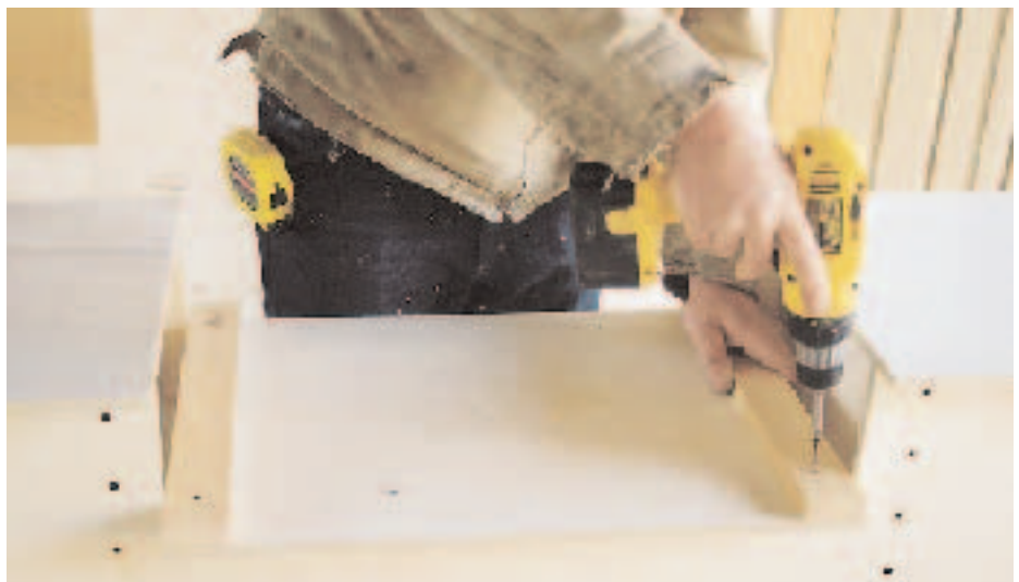
Figure 6. Shim strips precisely set the saw table height to the workbench.
