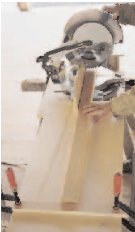
Figure 7. Clamped stops for productivity.
