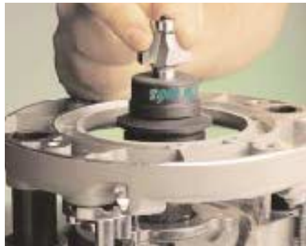
Figure 1. The PowerCollet replaces the existing collet on four brands of routers, eliminating the need for wrenches to change bits.
