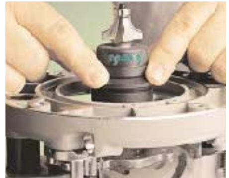
Figure 1. The PowerCollet replaces the existing collet on four brands of routers, eliminating the need for wrenches to change bits.
