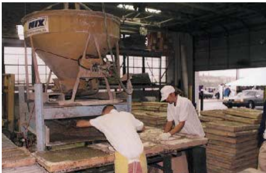
Figure 2. Manufactured stone is cast in molds made from natural stone. First, pigments are sprinkled into the molds (top), then the molds are filled with a cement mix (above). The filled molds are set on vibrating tables to get rid of bubbles.
