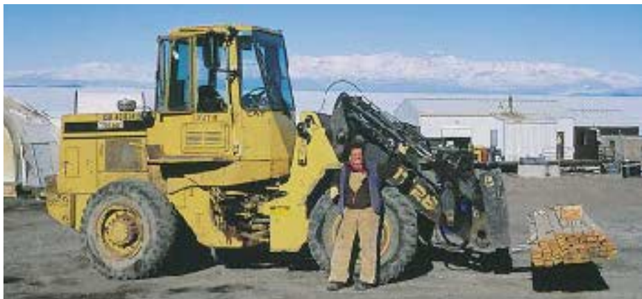
The author at McMurdo Station, Antarctica. Diesel engines are left running continuously to avoid difficult cold starts. On the other hand, round-the-clock summer daylight makes it possible to work outdoors at any hour.
