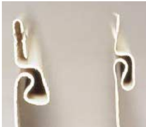
Figure 2. Several types of vinyl siding, including Alcoa's Grand Sierra, at left in photo, have a folded nail hem. These double-thickness hems are less likely to rip in a windstorm.
