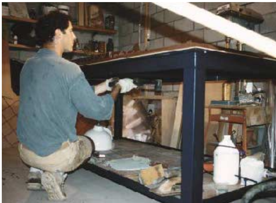
Figure 9. Vibration from the rhythmic pounding of a pair of rubber mallets settles the mix, driving out air bubbles to create a dense, solid mass and a smooth, void-free finished surface. Alternatively, the author uses electric vibrators, strategically mounted to his casting tables.
