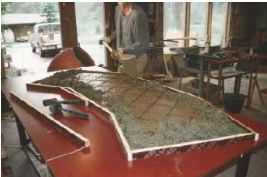
Figure 8. The author places the steel reinforcement after filling the forms two-thirds full. He uses colorized concrete to complete the perimeter of the casting and less costly, untinted concrete to fill in the field of the underside, which will not show. This ensures that the steel is properly located closer to the bottom of the counter, where it will best resist tension forces that may develop in service.
