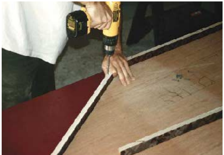
Figure 3. The author casts his pieces on a custom-built table that can be adjusted to dead level. After laying the template face-down on a sheet of ultra-smooth Finn Form plywood, which has a plastic release-film facing, the author surrounds it with sawn strips of form ply, screwing them to the base panel to create the casting form for the countertop section.
