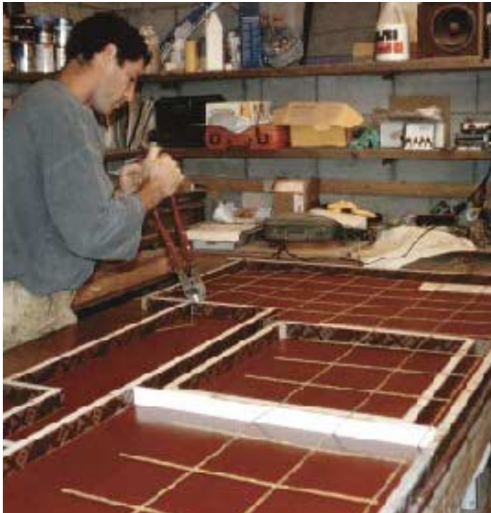
Figure 5. The author fabricates the reinforcement using wire cutters to drop an overlaid sheet of #9 wire mesh into the form. Narrow sections, such as the strip around a sink cutout, may be reinforced with a length of #3 rebar. Nylon cord, tied to the mesh, creates a lifting handle for moving the cured slab. After fitting, the steel is temporarily set aside.
