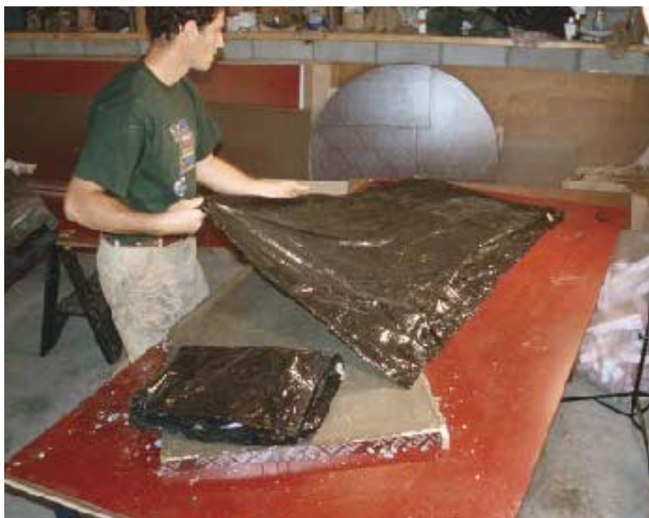
Figure 10. To slow water evaporation and prolong hydration of the cement, the casting is covered with poly and allowed to rest in the form for at least four days before removal.
