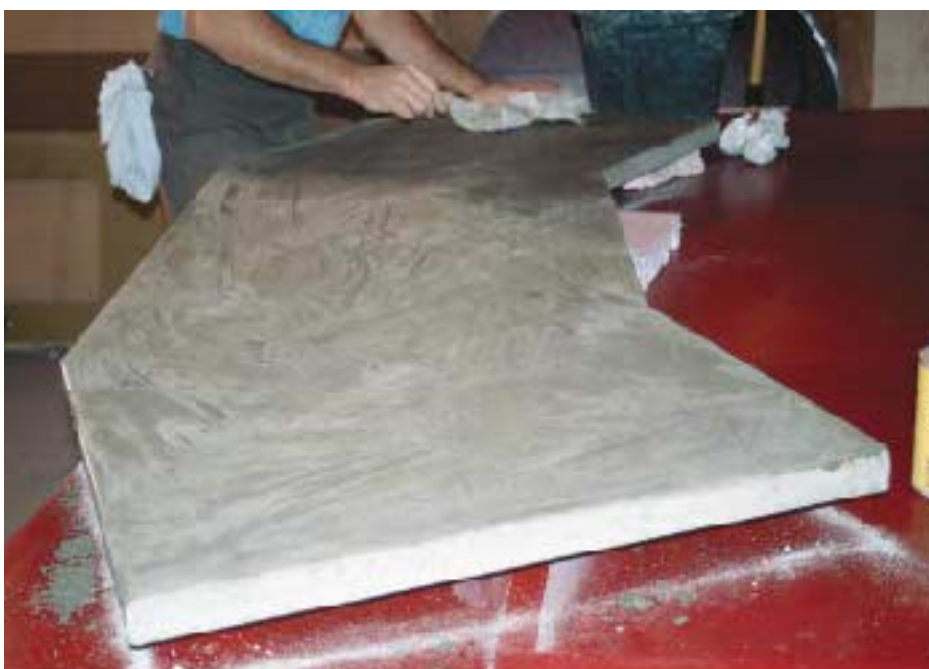
Figure 11. A few small pits and imperfections are always present in the surface of a countertop. The author has developed a special colorized grout mixture to rub and polish the surface, filling the voids and creating a flawless surface. Contrasting and complementary grout colors add to the complexity of a countertop's appearance.
