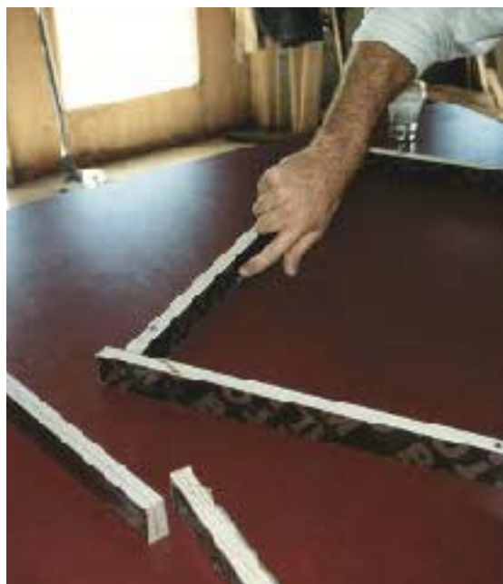
Figure 4. To eliminate any chance of the concrete sticking to the form, the author rubs a thin layer of release agent onto the form. Silicone caulk, applied to all inside corners and tooled smooth with a fingertip, imparts a subtle radius to the edge and corners of the cured concrete piece. The release agent also makes the silicone easy to peel away when the form is disassembled.
