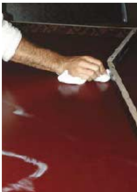
Figure 4. To eliminate any chance of the concrete sticking to the form, the author rubs a thin layer of release agent onto the form. Silicone caulk, applied to all inside corners and tooled smooth with a fingertip, imparts a subtle radius to the edge and corners of the cured concrete piece. The release agent also makes the silicone easy to peel away when the form is disassembled.
