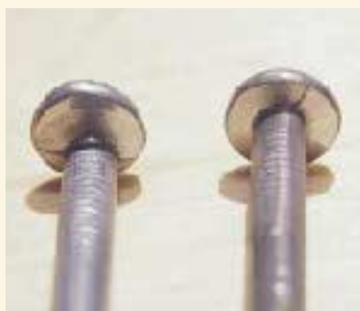
Figure 1. The offset head on these nails is designed to provide the close collation of clipped-head nails with more head-surface area and the finished appearance of a round-head (right). In the photo above are offset-head nails from Paslode, Senco, and Hitachi in two sizes: 2 3 / 8 x .113-inch, and 3 x .131-inch. A 12-penny sinker (above, far left) and standard round-head 3 by .131-inch pneumatic nail (above, far right) are shown for comparison.
