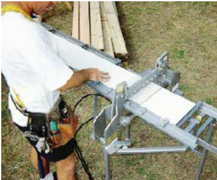
Figure 4. If you're a high-volume installer, the pneumatic Platform Shear and Roller Table are excellent, but too big for small jobs.
