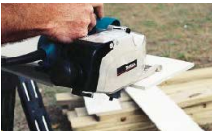
Figure 6. If you had to choose just one tool, the Makita 5057KB 110VAC, 7 1 / 4 -inch circular saw with dust collector (top) would be the one. The Makita 5044KB 4-inch circular saw with dust collector (bottom) is a compact saw that's as solid as the larger Makita, and will cut two pieces at once quite effectively.
