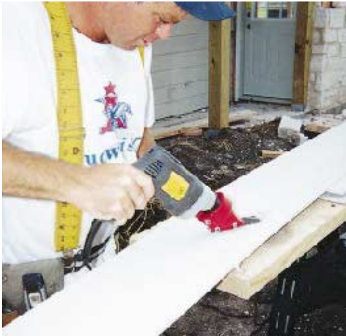
Figure 3. The SS306 WhipperSnapper is the best tool I've found for cutting curves.
