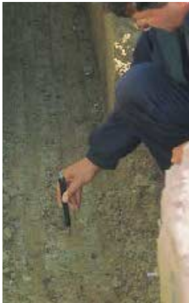
Figure 2. The author checks soil density in a footing trench using a penetrometer. Soil strength directly under the footing, where loads are concentrated, is crucial to foundation performance.
