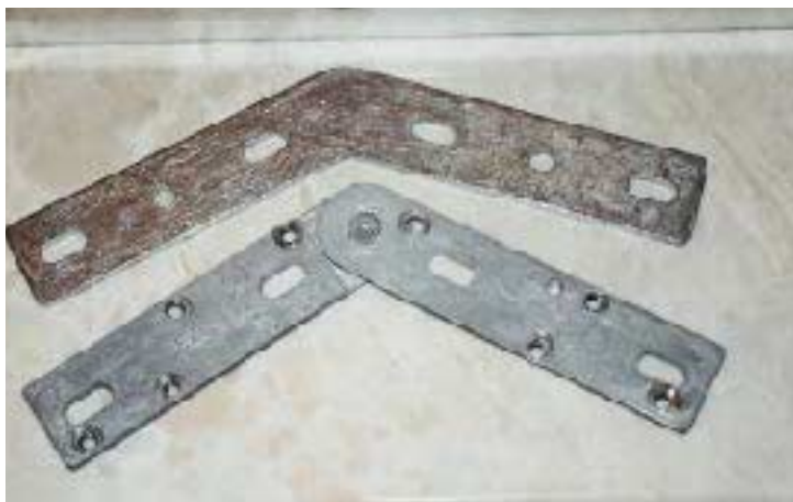
Figure 1. Head channel joining plates for frameless enclosures come in fixed corners of 90- and 135-degrees (left). Off-angles, which drive the cost of an enclosure up, are handled with an adjustable corner (above). The authors measure, cut, and join the extruded header sections on site.
