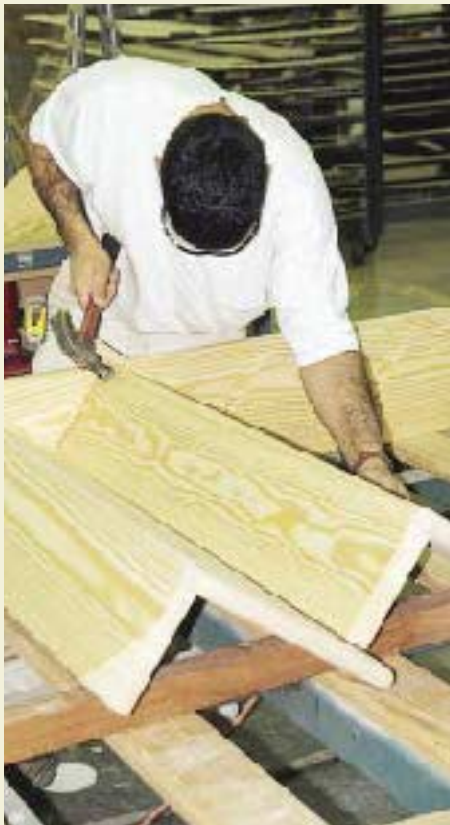
Figure 4. Stringers are precision-routed on a computer-controlled machine. The treads are securely wedged (left), glued (center), and screwed (right) in place.
