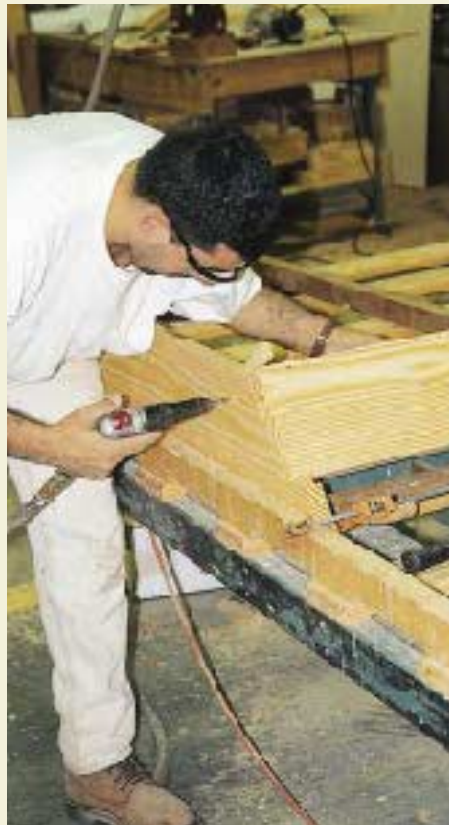
Figure 4. Stringers are precision-routed on a computer-controlled machine. The treads are securely wedged (left), glued (center), and screwed (right) in place.
