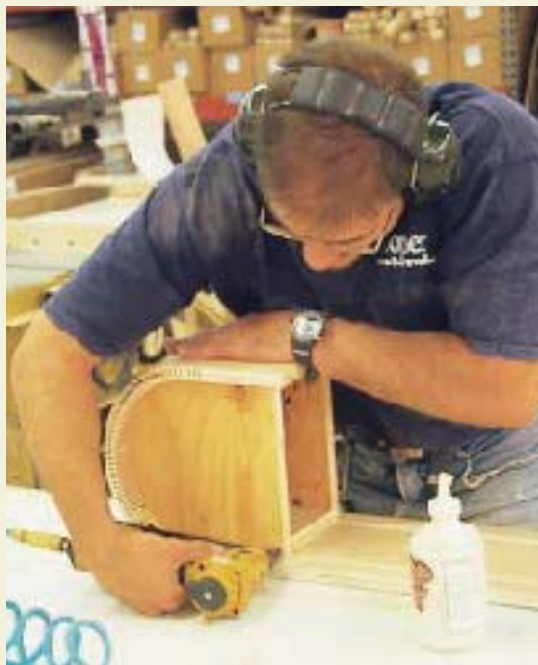
Figure 6. Kerfed plywood is bent around a pre-made form to make a bullnose riser.
