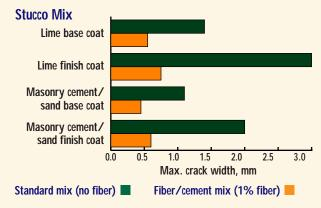
Some stucco plasterers use nylon or polypropylene fibers to reinforce the base coat of stucco. However, such fibers result in a hairy stucco that cannot be used for the finish coat. Unlike polypropylene fibers, cellulose fibers are invisible, even when used in the finish coat. "Polypropylene fibers are coarse fibers that don't disappear in the mix," says Parviz Soroushian, who conducted the research at Michigan State University. "Cellulose comes naturally in a very fine diameter."
