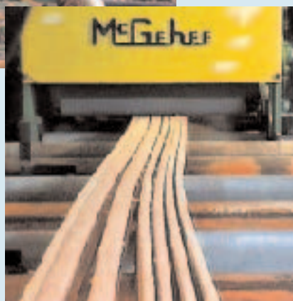
Curve sawing equipment, which is computer-controlled, allows the sawmill to follow the curve on an S-shaped log.
