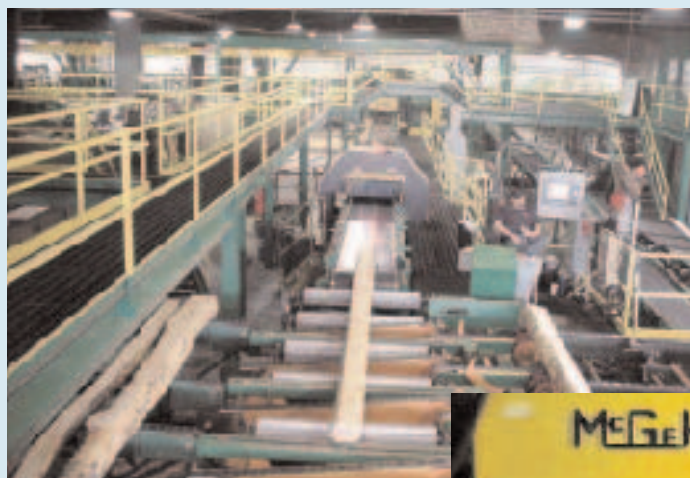
Curve sawing equipment, which is computer-controlled, allows the sawmill to follow the curve on an S-shaped log.
