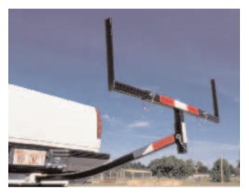
height and cargo widths between 27 and 49 inches, the square steel tubing breaks down for compact storage. Weighs 46 pounds, supports 750 lbs (don't exceed receiver rating), and comes with a snappy red caution flag, for around \$150.
