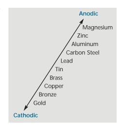
This chart ranks various metals from anodic to cathodic. A metal higher in the list can degrade when placed in contact with a metal that is lower.
