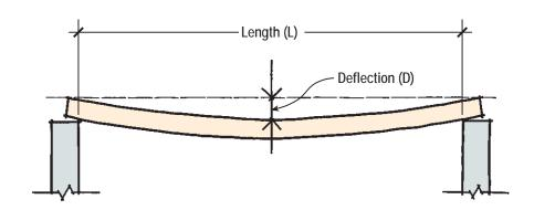
Maximum allowable deflection (D) for joists is equal to L/360For example, if L = 20'-0":
