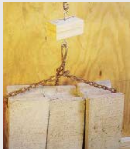
Figure B. The test blocks were suspended on a chain and gradually loaded with an increasing number of concrete blocks.
