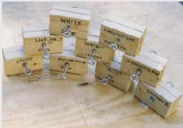
Figure A. Nine pairs of 2x4 blocks were fitted with eyebolts and glued together with different glues.
