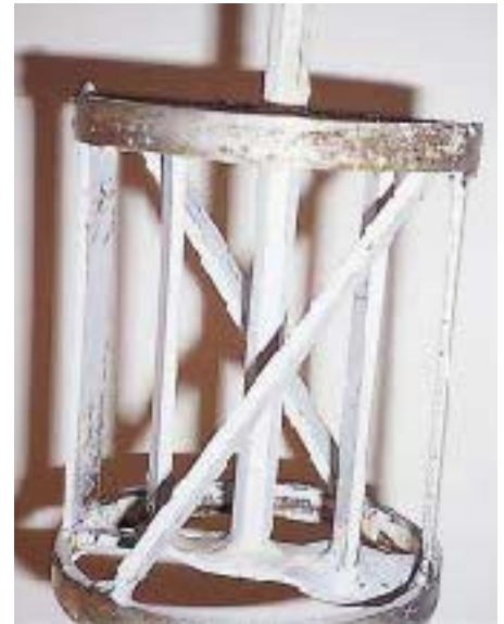
Figure 2. Tools of the plastering trade include a hawk and assorted trowels, a felt blister brush, miscellaneous paint brushes, and a spray bottle. A cage mixer (right) chucked in a low-speed drill ensures a smooth batch of plaster.
