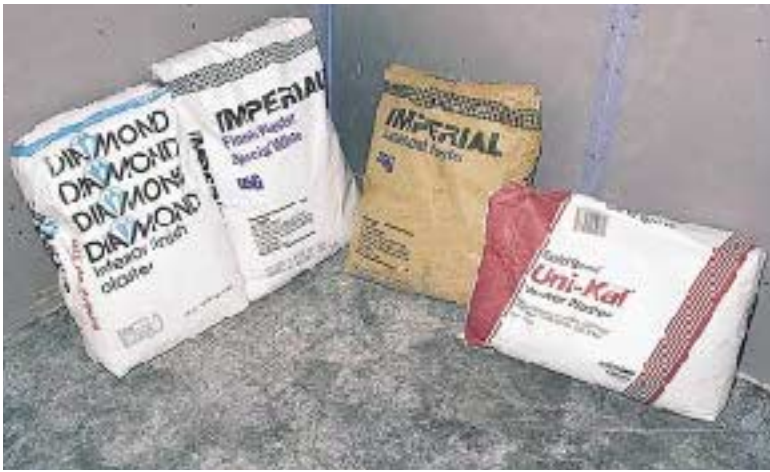
Figure 1. The most commonly used veneer plasters in southern New England are USG's Diamond and Imperial, and Gold Bond's Uni-Kal. Base-coat plaster is used in two-coat veneer systems. Imperial contains a fine aggregate that increases its compressive strength, but makes it more difficult to work with.
