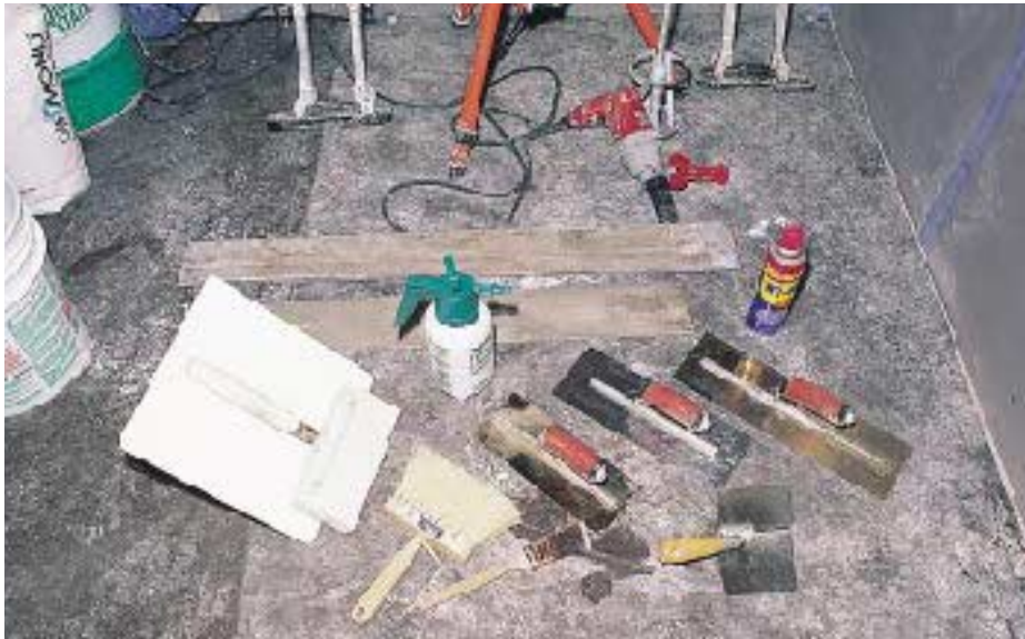
Figure 2. Tools of the plastering trade include a hawk and assorted trowels, a felt blister brush, miscellaneous paint brushes, and a spray bottle. A cage mixer (right) chucked in a low-speed drill ensures a smooth batch of plaster.
