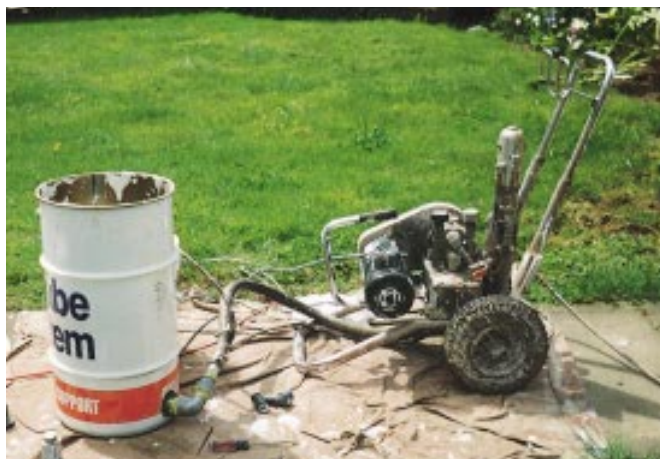
Figure 2. The author used a recycled grease drum, adapted for use as a container for the suction sprayer, to apply the heavy-bodied chemical paint stripper.
