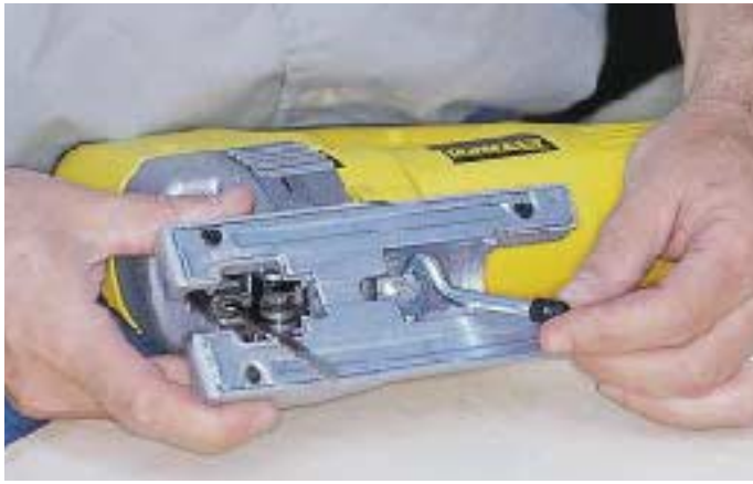
Bevel angle. Many of the new jigsaws come with no Allen wrench at all; even the bevel angle is adjustable without a tool. The DeWalt 321 (left) uses a pivoting lever on the base; the Porter-Cable 9543 has a rotating knob that folds down from the back of the saw (right).
