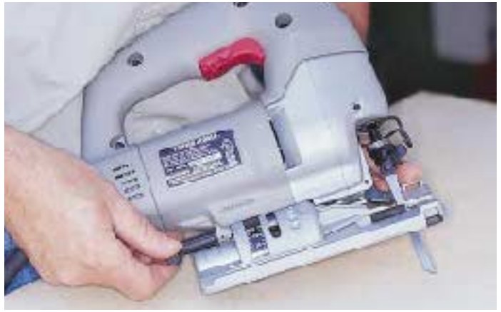
Bevel angle. Many of the new jigsaws come with no Allen wrench at all; even the bevel angle is adjustable without a tool. The DeWalt 321 (left) uses a pivoting lever on the base; the Porter-Cable 9543 has a rotating knob that folds down from the back of the saw (right).
