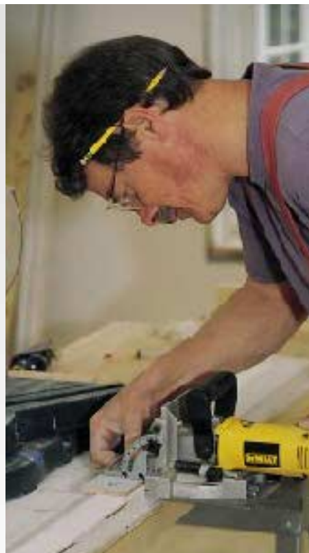
Using a spacer on half the cuts is a handy way to offset joints without resetting the fence.
