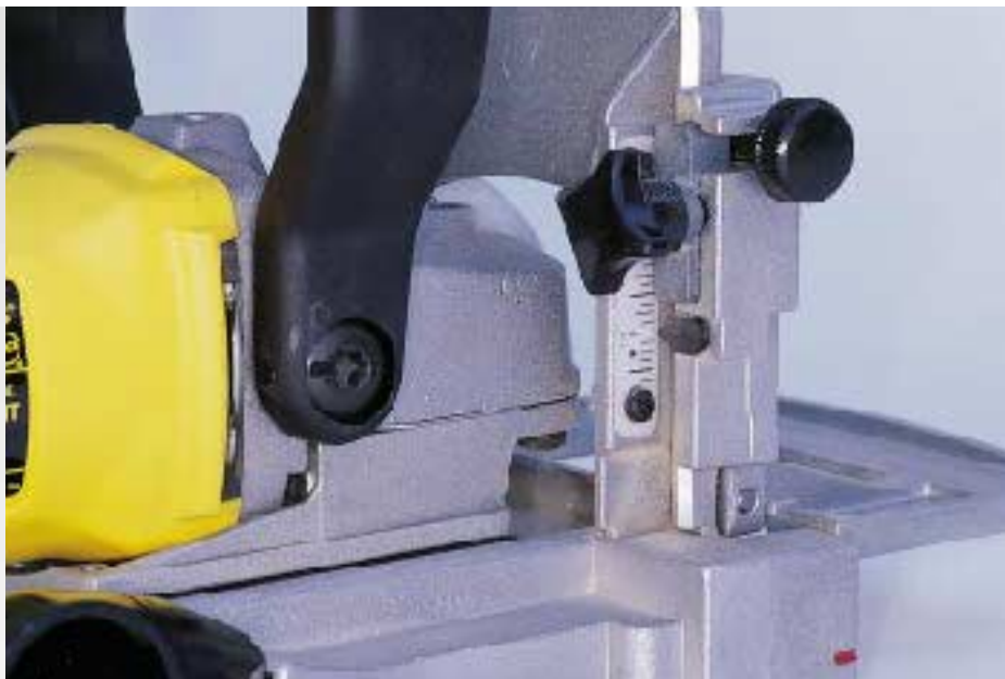
Scales are easier to read when the pointer is right up against the graduations.
