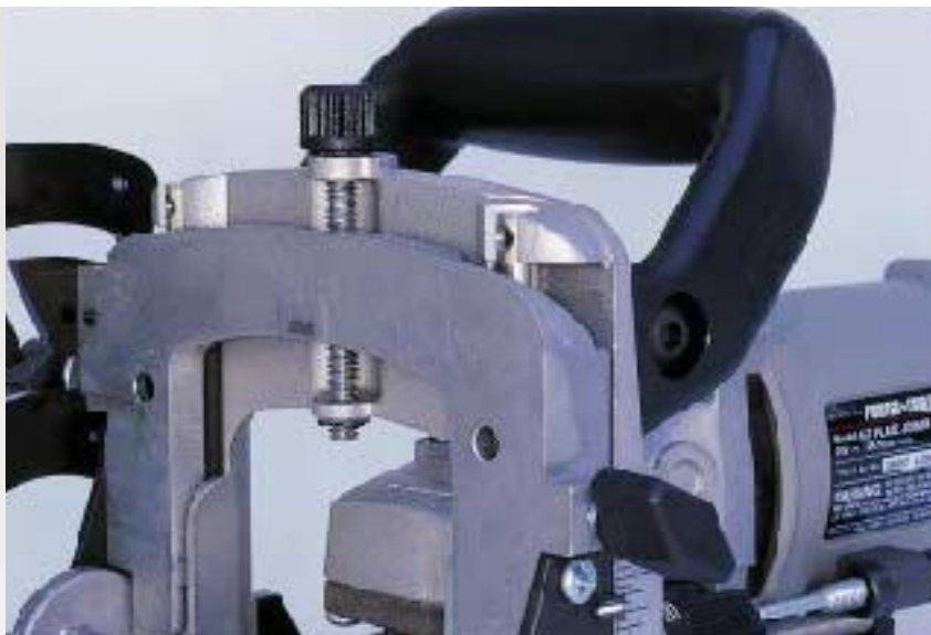
Porter-Cable uses a jackscrew mechanism to fine-adjust fence height.
