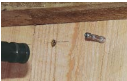
Figure 5. The collet on the Milwaukee will sometimes release if you bump it.
