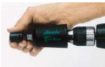
Figure 6. The Torq-Mate converts your electric drill motor into an impact driver. Impact sockets should always be used with any impact driver because regular sockets can break and cause injury.
