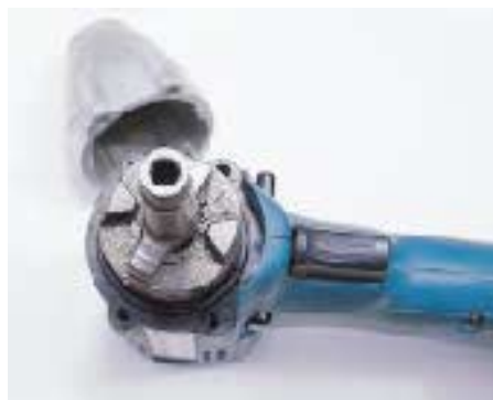
Figure 1. The rotational force of the motor is converted into intermittent force by the hammer and anvil arrangement inside the nose of the tool (left). A spring allows the mechanism to release at a preset value (right). This intermittently resolved force is where the extra power comes from — just like hitting a wrench with a hammer to loosen a nut.
