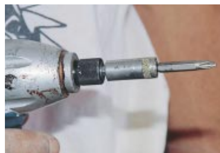
Figure 2. Any 1/4-inch hex-drive accessory will fit, so you have lots of choices.
