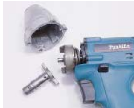
Figure 1. The rotational force of the motor is converted into intermittent force by the hammer and anvil arrangement inside the nose of the tool (left). A spring allows the mechanism to release at a preset value (right). This intermittently resolved force is where the extra power comes from — just like hitting a wrench with a hammer to loosen a nut.
