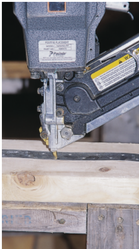
Figure 3. The brass-coated titanium probe at the tip of the Paslode Positive Placement nailer makes it easy to locate the nail holes in metal hangers. The probe pivots out of the way as the nail is driven.
