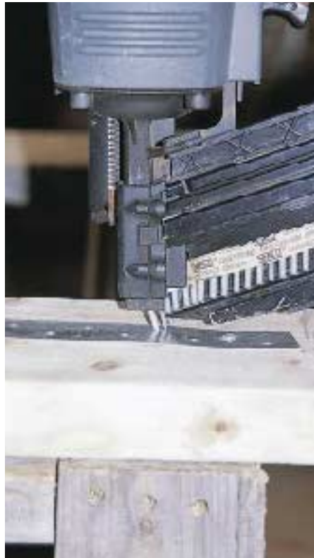
Figure 4. When using the Senco nailer, it's important not to push the gun forward or else the nail will not fire straight.
