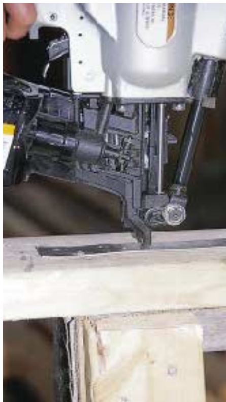
Figure 2. The Max CN601J coil nailer holds 100 hanger nails at a time. The location of the safety release arm alongside the nail (left) makes it tricky to see and place the nail when working lefthanded.
