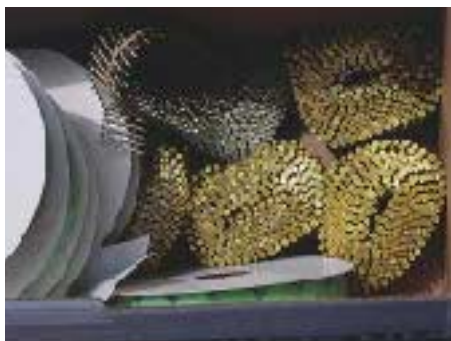
Figure 4. The only problems the author had with the Plasti-Tacker Pro were the result of collation. The nail coils shown here were bent during shipping, causing jams.
