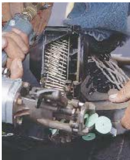
Figure 2. The plastic caps are automatically fed down a track to the nose of the coil nailer.
