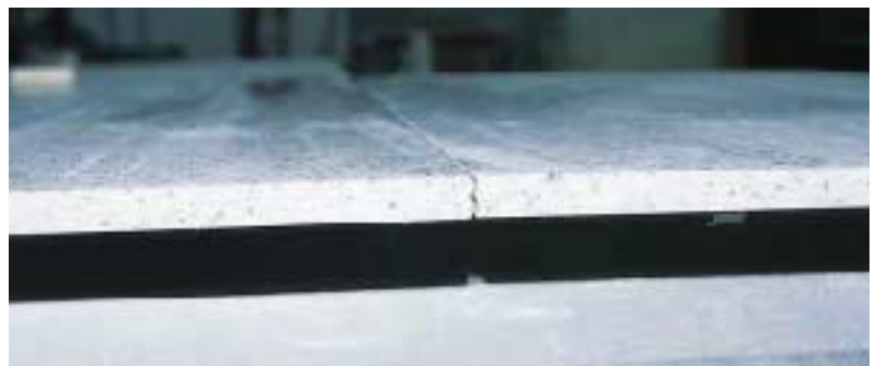
Figure 9. A wavy router bit (top) creates an edge with more surface area for gluing. The key to using a wavy bit is the special stepped router base. The first cut is made with the high side of the base riding on the material. Then the second piece of solid-surfacing is cut using the low side of the base. The offset in the router base heights allows the two pieces to mate, leaving the top surfaces on the same plane. The resulting joint (above) forms a curvy version of a tongue-and-groove joint.
