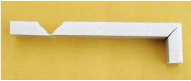
Figure 5. A V-grooving machine is a type of automatic router that can cut a V-groove with great precision. The cut is backed up with tape that becomes a hinge when the solid-surfacing is folded and glued, forming a miter joint.
