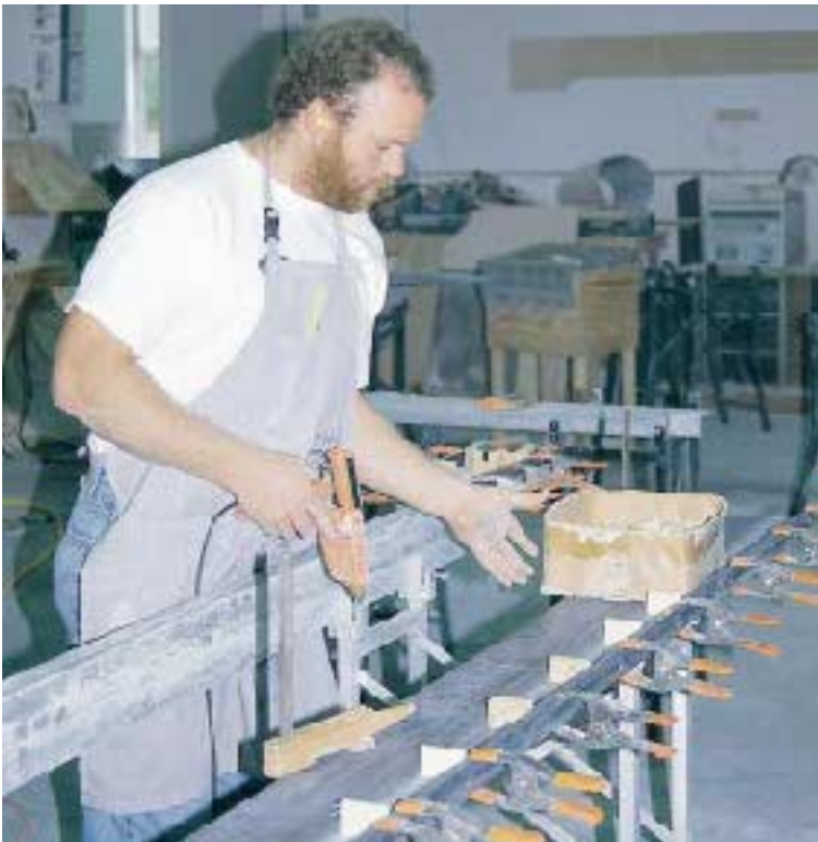
Figure 7. Before gluing the solid-surface strips used to build up a countertop edge, small blocks of plywood are attached to the top with hot-melt glue. These blocks act as stops to prevent the glued strips from sliding around while being clamped.
