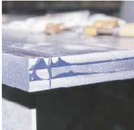
Figure 6. Most solid-surface countertops are only \frac{1}{2} inch thick, so fabricators build up the exposed edge with extra material to make the top appear thicker. Gluing up an edge takes dozens of spring clamps (far left). After a pass with a router equipped with a straight bit, the seams on a built-up edge almost disappear (left).
