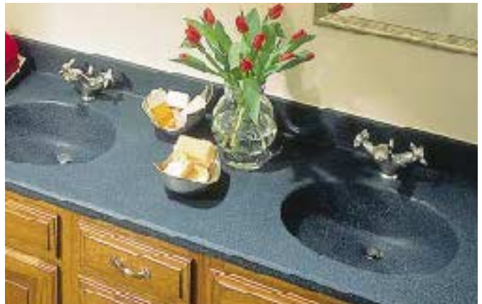
Figure 4. Several manufacturers offer pre-formed lavatory tops, eliminating the need for fabrication. This two-bowl top from Transolid is manufactured by thermoforming. Transolid also sells lavatory tops with undermount sinks that have been factory-seamed to the counter.
