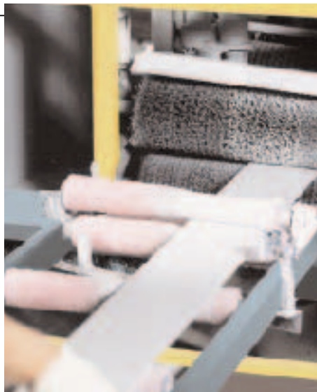
Figure 1. As a piece of siding is pulled through a machine coater, it is flooded with paint (left). On the other side of the machine, rollers or brushes remove the excess paint (right).
