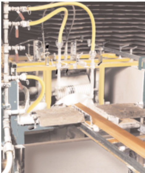
Figure 1. As a piece of siding is pulled through a machine coater, it is flooded with paint (left). On the other side of the machine, rollers or brushes remove the excess paint (right).
