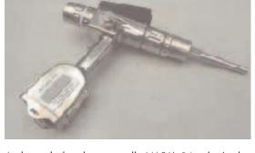
At the end of each spacewalk, NASA's 24-volt pistolgrip tool, or PGT, can be linked to an on-board computer, which downloads and records the number of turns and degree of torque delivered to each bolt. Tightening fasteners in zero gravity takes some experience: Unless the astronaut remembers to clip into a restraint system before squeezing the trigger, both user and tool may find themselves revolving freely around a stationary bolt.
