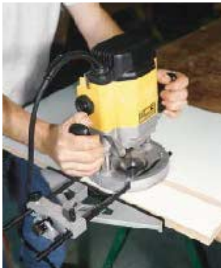
A fence is essential for many milling operations. Fences range from simple but effective edge guides (above left) to Festool's aluminum rail system, which makes long straight cuts easy (above right).
