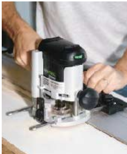
A fence is essential for many milling operations. Fences range from simple but effective edge guides (above left) to Festool's aluminum rail system, which makes long straight cuts easy (above right).
