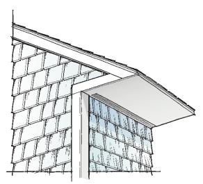
Do away with the eaves fascia board altogether for a modern approach that looks best with a steep roof and an overhang of 30 inches or more.
