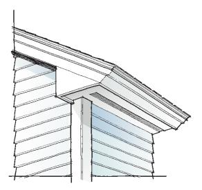
Replacing the flat eaves fascia with a sloping one gives a more contemporary look that's appropriate where more shading is needed.
