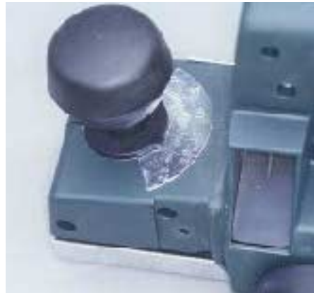
Indexed detents make it easy to keep track of how much material you're about to remove.
