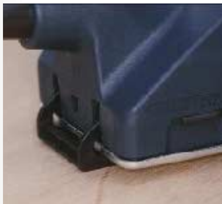
A parking foot, standard on many planers, allows you to set the tool down without waiting for the blades to stop turning.
