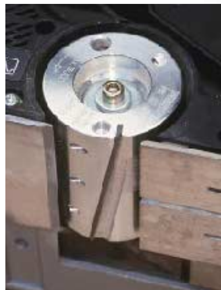
Festo's spiral cutter uses a single removable carbide blade.
