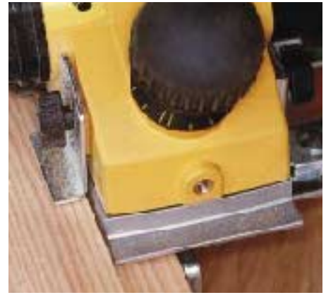
Most power planers can be used to cut rabbets on the edge of stock. The fence is used to set width of cut, and the rabbeting stop determines depth.
