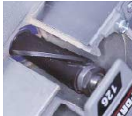
The Porta-Plane has a two-blade spiral cutter that can be removed for sharpening.
