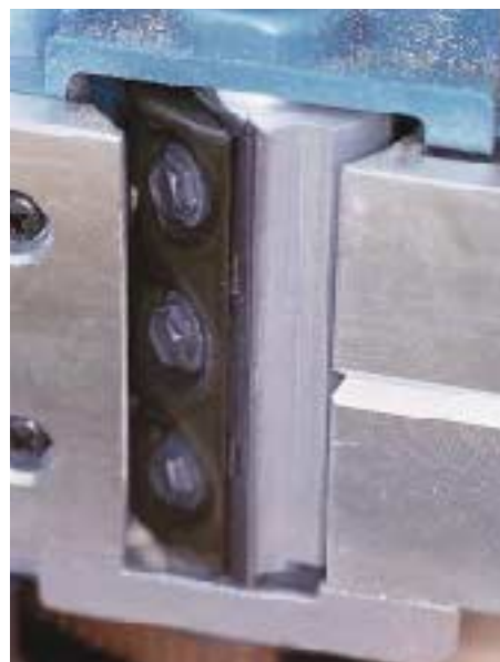
Some manufacturers use bolts to fasten the blades directly to the head (above), while others use blade holders that fit into slots in the head and are secured with Allen screws (right).
