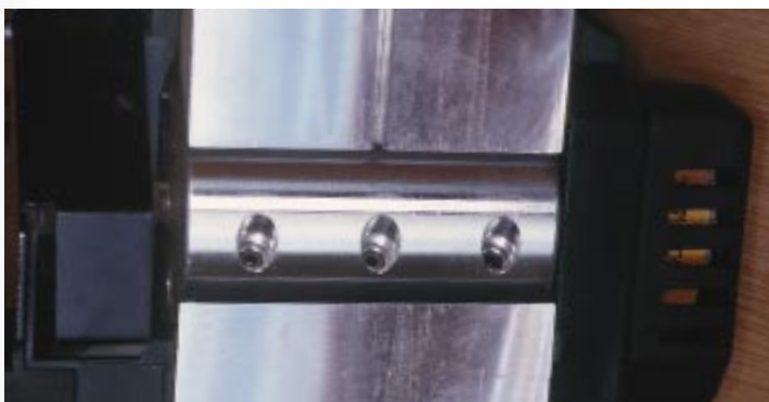
Some manufacturers use bolts to fasten the blades directly to the head (above), while others use blade holders that fit into slots in the head and are secured with Allen screws (right).
