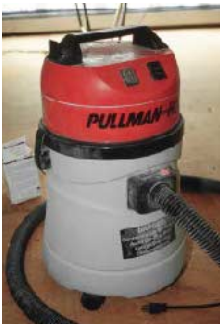
Figure 7. Each job has its own ten-gallon HEPA vac. Unlike that of an ordinary shop vac, its exhaust is almost entirely free of even the tiniest dust particles. Because the used vacuum bags and filters may contain lead dust, they are considered low-level hazardous waste.
