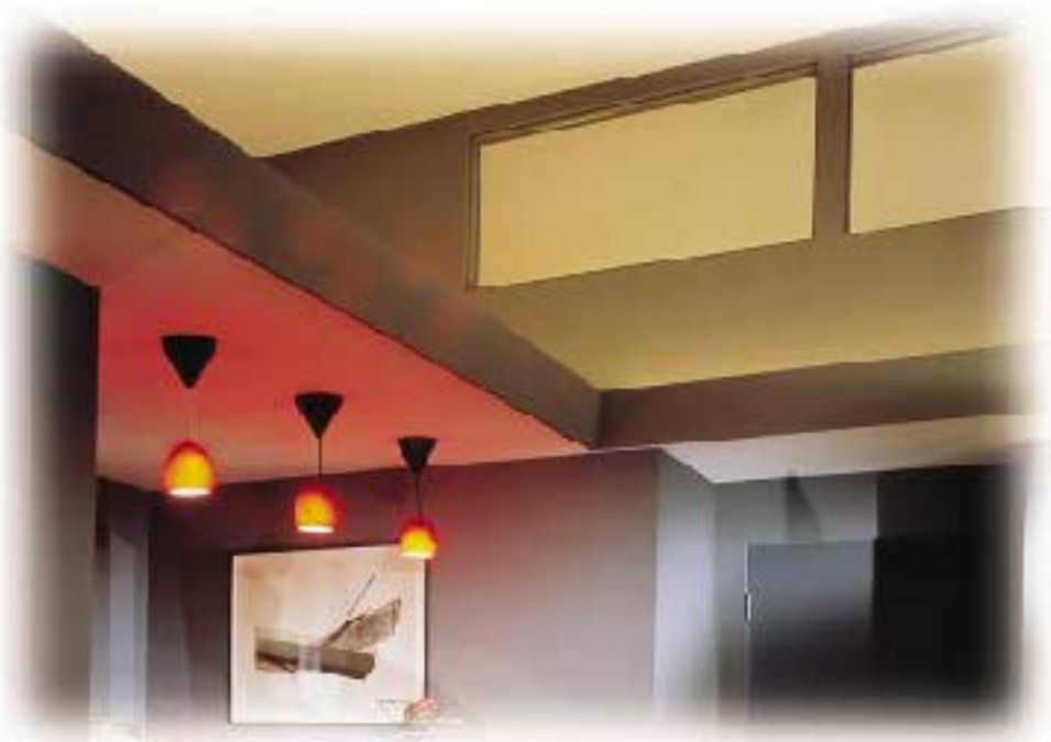
Figure 4. The ambient light in this room is provided by cove lighting mounted above the ledge and cantilever.
