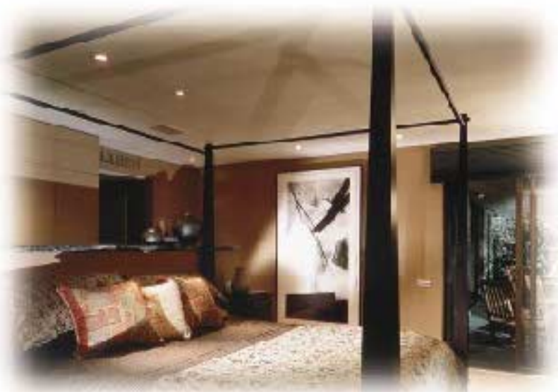
Figure 9. A pair of separately switched, recessed ceiling fixtures over the bed provide reading lights for two people. The light on the right is aimed at the left side of the bed and vice versa, so that one person can read and the other can sleep without getting light in their eyes.
