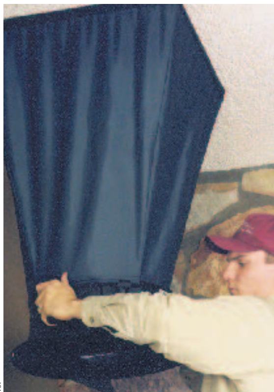
Figure 3. An airflow hood (left) measures the airflow at a supply register or return grille in cfm. If the register is in a difficult-to-access location, a funnel-like device, TSI’s Air Flow Horn (above), can be used in conjunction with a hot-wire anemometer to measure airflow.
