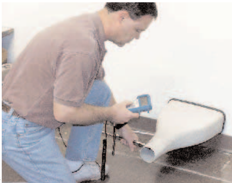
Figure 3. An airflow hood (left) measures the airflow at a supply register or return grille in cfm. If the register is in a difficult-to-access location, a funnel-like device, TSI’s Air Flow Horn (above), can be used in conjunction with a hot-wire anemometer to measure airflow.
