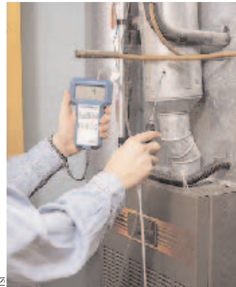
Figure 6. A flue gas analyzer, like the CombuCheck from TSI, measures levels of oxygen and carbon monoxide in the flue gas of a combustion appliance.
