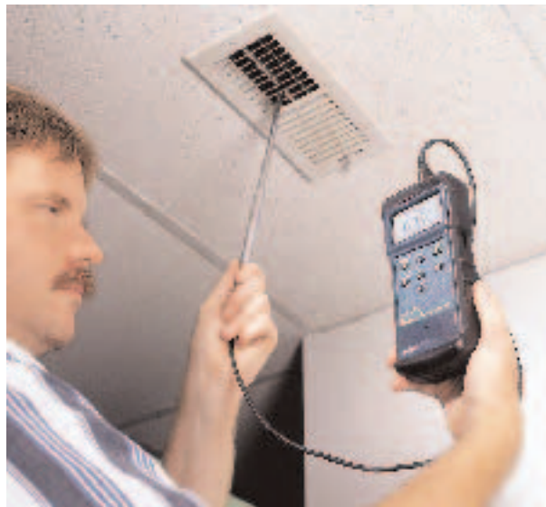
Figure 4. When an airflow hood is unavailable, or in locations where an airflow hood cannot be used, airflow can be measured with a hot-wire anemometer. Most hot-wire anemometers, like this model 407123 from Extech, can record both air velocity and air temperature.
