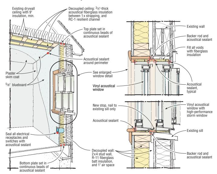
**Figure 8.** Double wall and ceiling construction decouples, or isolates, the interior space from the exterior building envelope. Although the existing room size is slightly reduced, the thunder of a passing jet is lowered to background noise.
