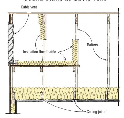
**Figure 6.** Roof vents provide a potential path for noise entry. A custom insulation-lined baffle disrupts and muffles sound entering the structure.
