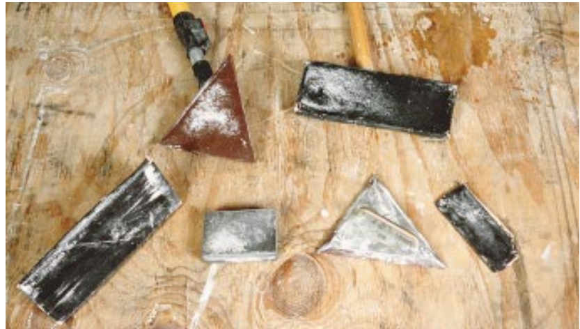
Figure 14. A sanding screen or 150-grit sandpaper is the best choice for finish sanding (left). Screens can be flipped over when the abrasive is worn. The author uses a variety of pole-mounted and hand-held sanders (right). Triangular sanding heads are particularly useful in corners.
