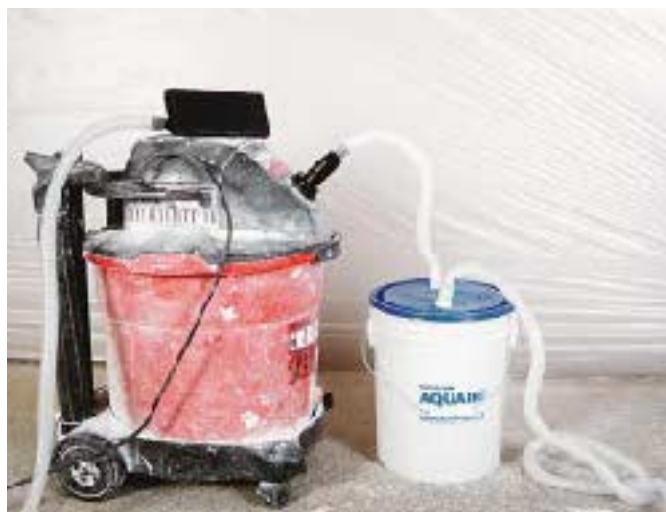
Figure 15. This dustless attachment for a shop vacuum captures nearly all of the sanding dust in a water filter (left). A temporary dust curtain is useful on remodeling sites (above).
