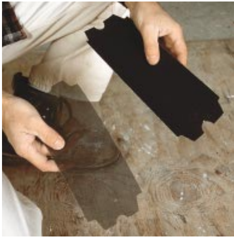
Figure 14. A sanding screen or 150-grit sandpaper is the best choice for finish sanding (left). Screens can be flipped over when the abrasive is worn. The author uses a variety of pole-mounted and hand-held sanders (right). Triangular sanding heads are particularly useful in corners.
