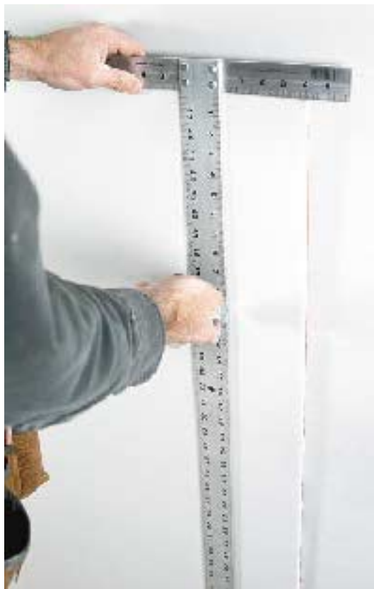
Figure 1. This pro-duty T-square from Warner has a 1/4-inch-thick tongue (left); most lumberyard varieties have only 1/8-inch-thick tongues. Graduated notches on the Johnson 24-inch ripping square guide make it easy to use a utility knife for long cuts (above).
