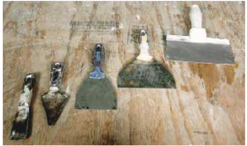
Figure 9. The author's main tapping knife has a 6-inch-wide blade, but he keeps other sizes and shapes handy for tight corners and spaces. Stiffer blades are best for the first, tape-embedding coat, while more flexible blades are best for smoothing finish coats.
