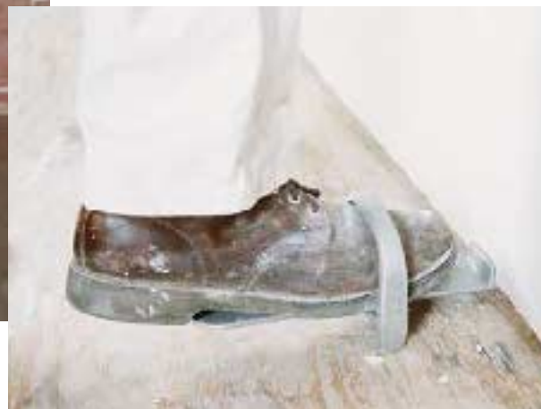
Figure 6. A foot lift works like a small lever to boost lower wall panels into position, leaving both hands free for fastening.
