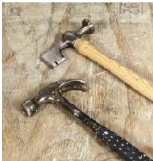
Figure 7. Unlike a carpenter's hammer, the convex face on a drywall hammer makes a dimple in the panel without tearing the paper facing. The hatchet-like blade is used mostly for prying.
