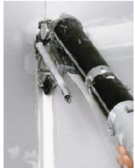
Figure 17. Mechanical taping tools must be loaded with compound using a special pump (left). Attachments adapt the pump to various finishing tools.
