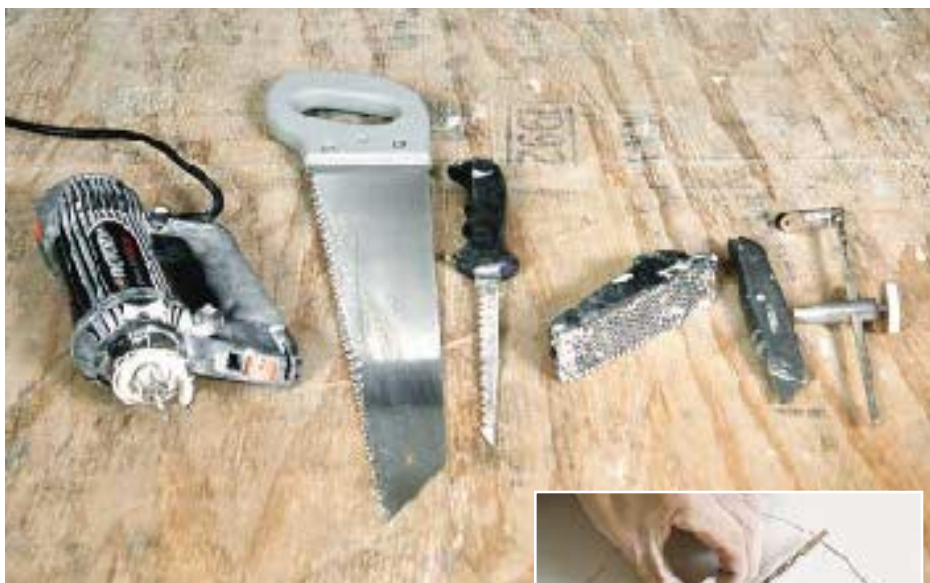
Figure 2. The author's cutting tools include (above, left to right) a drywall router, a wide-blade drywall saw, a keyhole saw, a pocket rasp, a utility knife, and a calibrated circle cutter (right).
