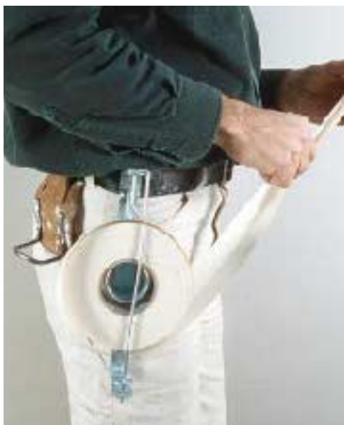
Figure 12. A tape roll keeps up to 500 feet of paper tape handy on a belt-mounted dispenser.
