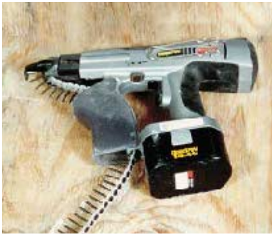
Figure 8. Although he often uses a standard electric drywall screwgun, the author also likes the convenience of the Senco cordless self-feeding screwgun.
