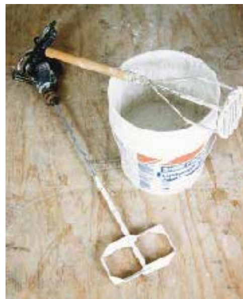
Figure 13. A hand mixer loosens up ready-mix, while a drill-mounted paddle mixer takes the drudgery out of mixing dry setting-type compounds.
