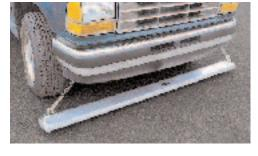
penny nail from 5 inches off the ground. The recommended suspension height is between 2 and 4 inches from grade. Once the magnet is full of nails, just sweep them off with a gloved hand. The MRS78 hang-type sweeper magnet is 78 inches long and costs \$375.
