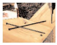
spikes, which require predrilling and are slow to drive. FastenMaster TimberLok screws, which come in five sizes up to 10 inches long, can be driven through pressuretreated beams with no predrilling. The screws are also handy for attach-
