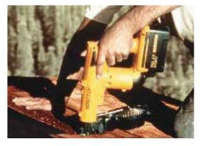
delivers a series of blows — 8 to 10 blows per nail — to drive the nail home.
