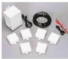
connects each illuminated paver to the light source, an illuminator. The illuminator requires 120 volts AC, and must be located within 40 feet of the pavers. One illuminator can serve up to 18 paver fixtures.
