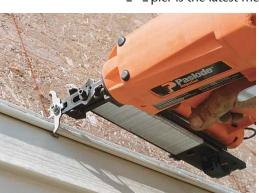
ples with a small internal combustion engine (fueled with MAPP gas and ignited by a spark from a Ni-Cad battery), no pneumatic hose or compressor is necessary.
