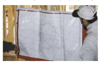
prints. Blueprint pages are slipped individually into sturdy transparent pockets and held in place with Velcro closures. Each pocket of the Plan-Caddy can be flipped, so that it reads like a book. The Plan-Caddy includes an extra pocket for information like window schedules or truss layouts. The standard size Plan-Caddy (for 24x36-inch prints) holds 5 pages, and costs \$98.50.
