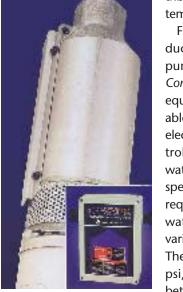
Flint & Walling has introduced a new submersible pump, the stainless-steel Commander Pro. This pump is equipped with a Franklin variable-speed motor and a special electronic controller. The controller senses the domestic water pressure and adjusts the speed of the pump motor as required to maintain a steady water pressure that never varies more than 1 or 2 psi. The controller is preset to 40 psi, but can be adjusted between 20 and 65 psi.
