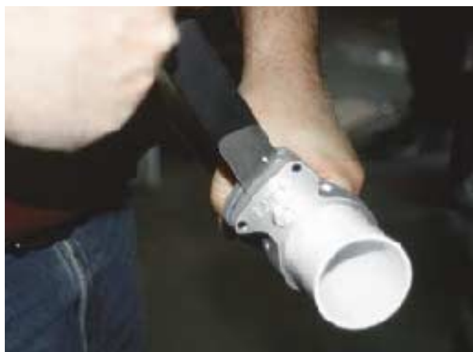
Figure 2. A thin-wall tubing cutter ensures clean, burr-free cuts for unimpeded airflow within the tubing.
